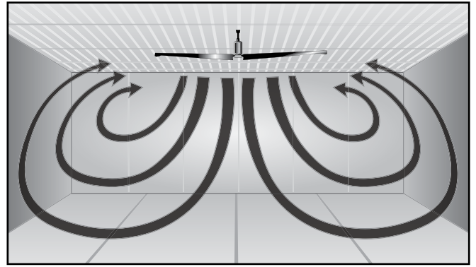
Area with an even room temperature after destratification.
